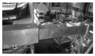
2. Install the bracket on bottom side and insert the two M10 bolts in the M11 holes.
