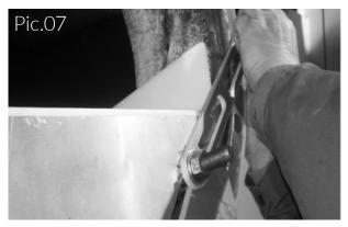
4) After fixing wing extensions use two bolts M16 to mount RS on the flange. After that, all bolts must be properly tightened. (pic.8). Bolts size depends on flange thickness.
