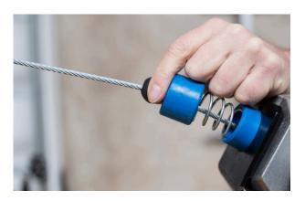
To avoid the cable beeing stuck in guide make sure it reaches the slider in the correct position.
